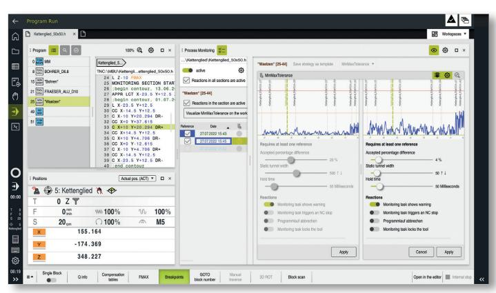
The Component Monitoring software option of the TNC7 protects your valuable machine tool assets. It's a toolbox that allows machine manufacturers to implement extensive monitoring functions. During machining, this function can protect the spindle bearing from overload, detect growing component wear in the drive train, and more.
