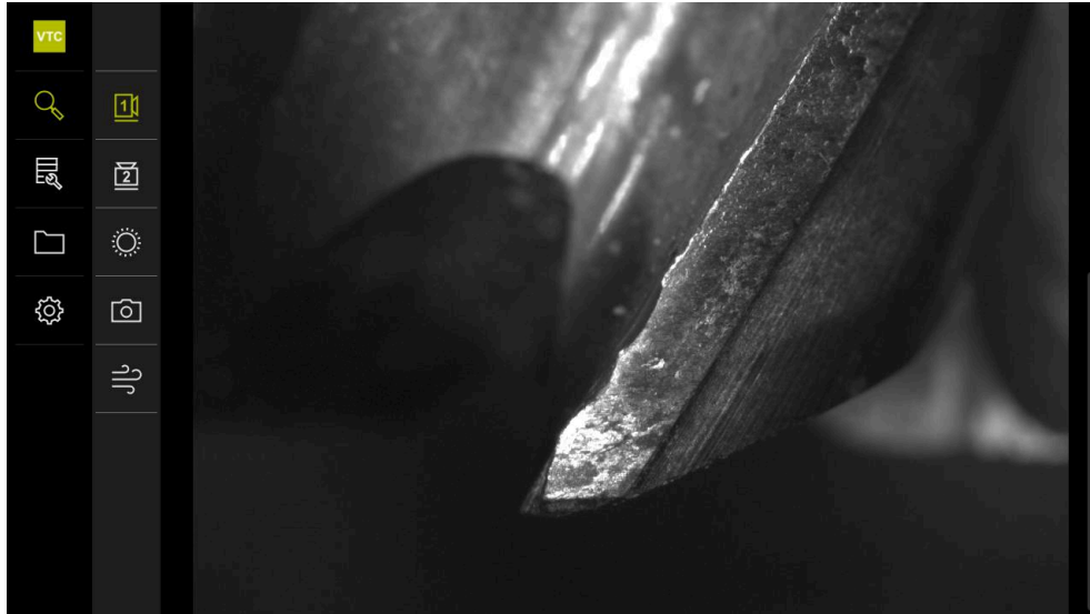
Figure 8: Manual tool inspection menu
