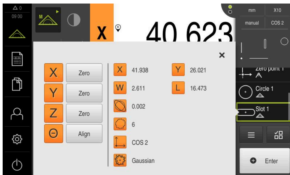
Figure 20: Slot feature in the feature list with Measurement result preview
