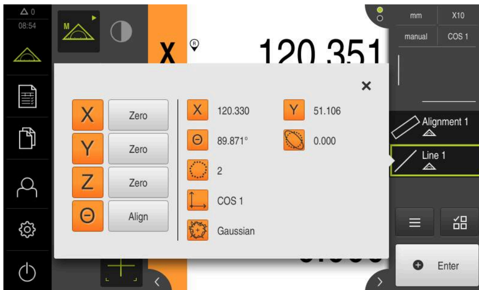
Figure 16: Line feature in the feature list with Measurement result preview
