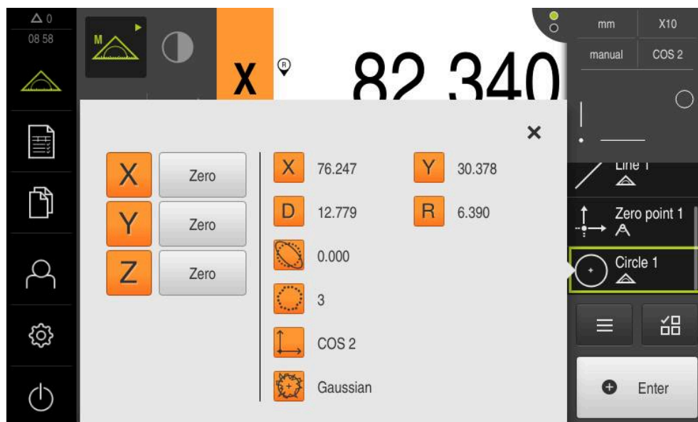
Figure 19: Circle feature in the feature list with Measurement result preview
