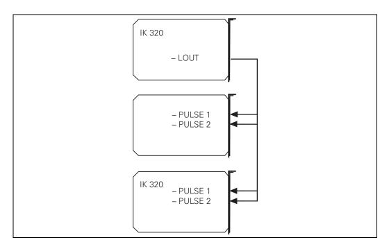
**8.1.7 VMEbus Indirect Latching**A local interrupt on the IK 320 is generated by an ADO access to the interrupt address of address space A16. The CPU performs the function set in parameter P81: the functions \$01, \$02, \$03 generate a latch signal in the corresponding axes.
