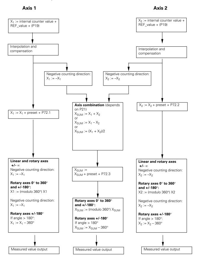
The REF value is the absolute value of the first traversed reference mark on encoders with distance-coded reference marks. On encoders with only one reference mark the REF value = 0.
