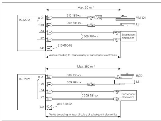
\*For 5.1-V power supply and current consumption of the encoder < 65 mA.
