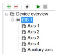
Click to select the respective EIB or axis. The selection of an EIB or an axis determines which tabs are shown/hidden in the EIB functions.
