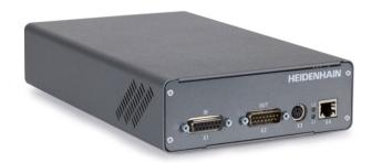
Mounting wizard for modular inductive rotary encoders with EnDat22 and direct outputting of the "Mounting clearance" mounting parameter
