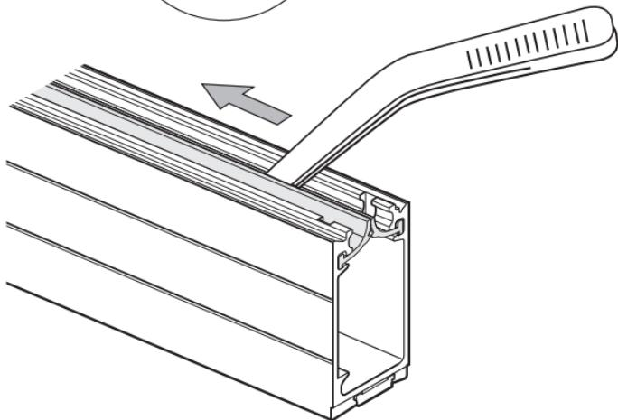
Carefully insert the exchange scanning unit. Avoid contact between the scanning reticle of the scanning unit and the glass scale!
