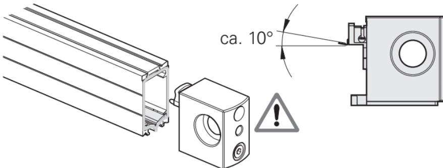
The end blocks are assigned specifically to the scale ends. Do not interchange, as this can result in damage to the scanning.
