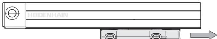
If the interior is contaminated, the sealing lips should be removed. The sealing lips can be used again.
