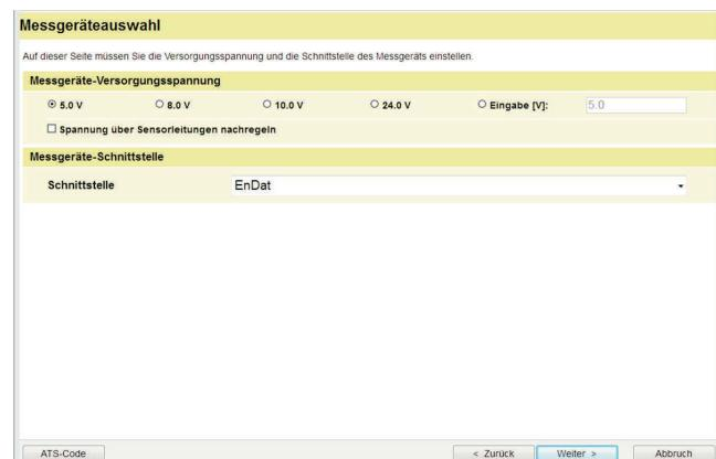
The following ATS code is to be entered for setting up a manual connection between the scanning head and the ATS software (not with EnDat 3):
