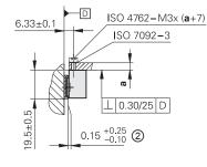
mm  $\Box$ Tolerancing ISO 8015 ISO 2768 - m H < 6 mm: ±0.2 mm
