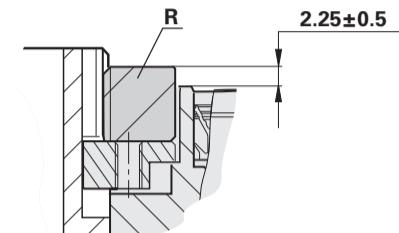
**Front-end shaft coupling (with mechanical fault exclusion).**
