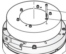
**Shaft coupling with ring nut [R] (without mechanical fault exclusion)**
