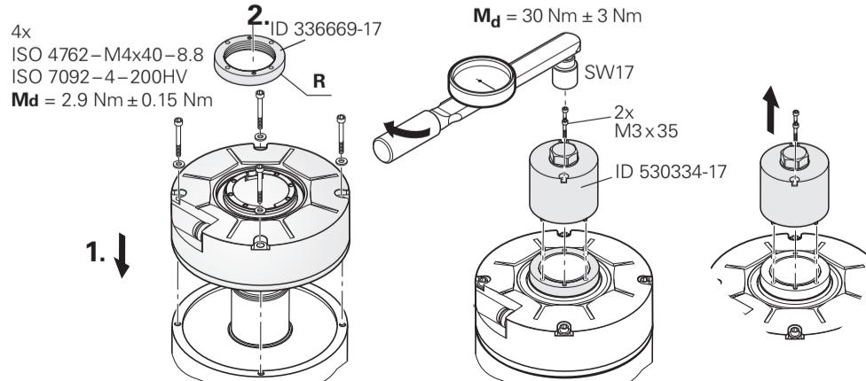
**Front-end shaft coupling (without mechanical fault exclusion)**
