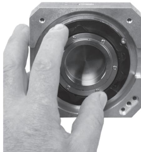
Check the resistance between the flange socket, rotor **a)** and stator mounting screw **b)**. Nominal value: < 1 ohm
