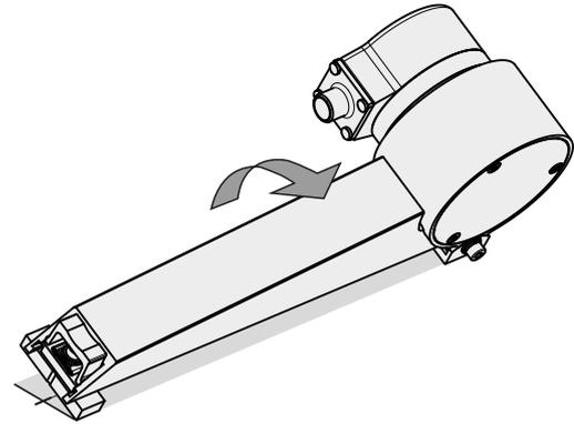
Connect an additional grounding conductor at the provided connection. The grounding conductor must be connected with an M4 screw and washers in their original sequence.
