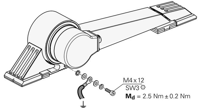
To ensure the listed minimal distances from sources of interference, use only HEIDENHAIN components (sensor, cabling, downstream electronics).
