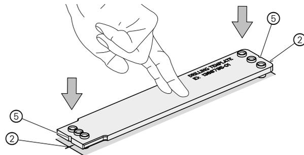
▶ First hole ⑥ Ø5 mm; drill >20 mm deep, insert the fixing screw with anchor, and fasten the mounting kit.
