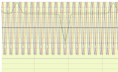
Figure 42: Complete reference pulse including quiescent value and usable component
