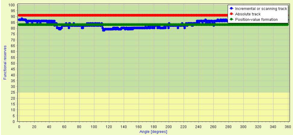
Figure 106: X/Y display of the Online diagnostics function
