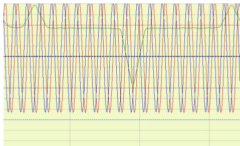
Figure 33: Complete reference pulse including quiescent value and usable component
