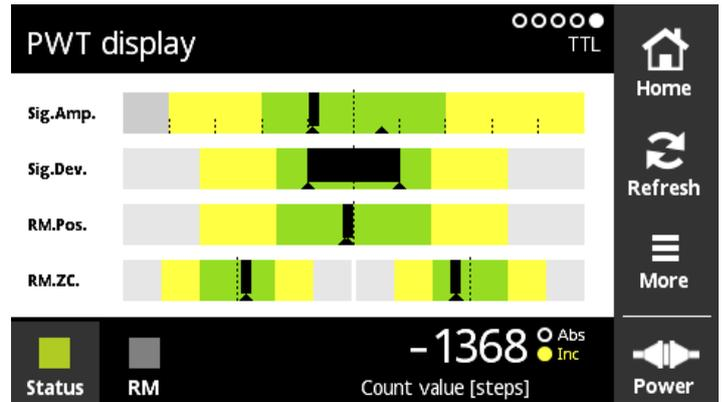
Then traverse the entire measuring length. All four bars must be in the green area; otherwise check the mounting tolerances.
