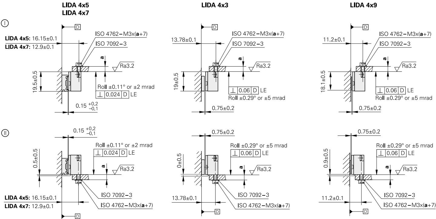
When you use mounting option ⑩, you can use the blind hole in the scanning head for adjusting the scanning head.
