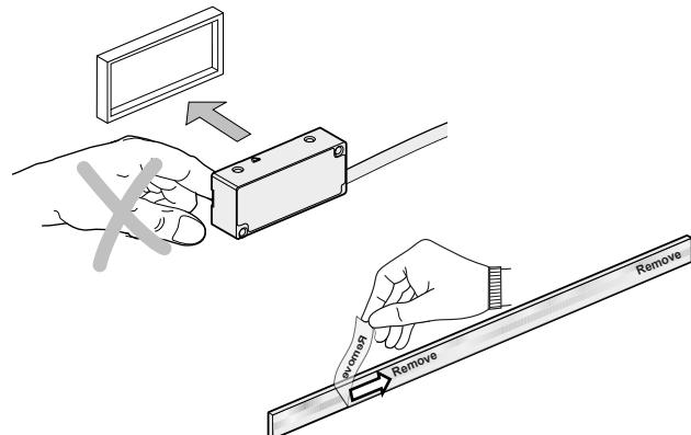
If necessary, clean the graduation and the scanning head with a lint-free cloth and isopropyl alcohol.
