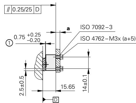
① = Mounting clearance between the scanning head and graduation
