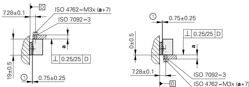
① = Mounting clearance between the scanning head and graduation
