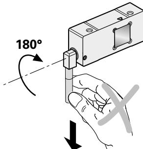
Do not pull the cable! This may cause damage to the cable.
