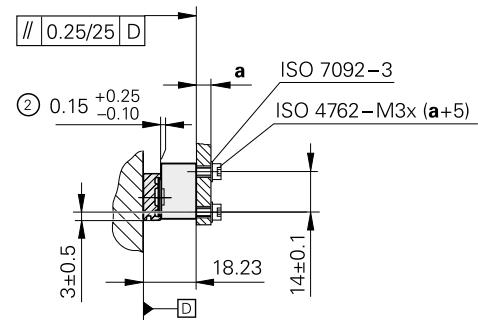
② = Mounting clearance between the scanning head and scale tape carrier
