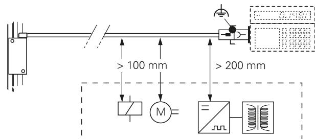
Note the maximum permissible pivot range of the adjustable cable outlet. Exceeding the pivot range may damage the scanning head! The cable may be rotated no more than a few times ( $\leq 10$ ), because otherwise proper functioning will be impaired.
