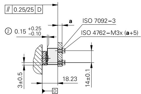
(2) = Mounting clearance between the scanning head and scale tape carrier
