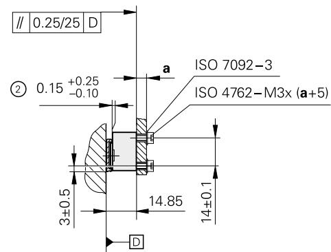
(2) = Mounting clearance between the scanning head and scale tape carrier
