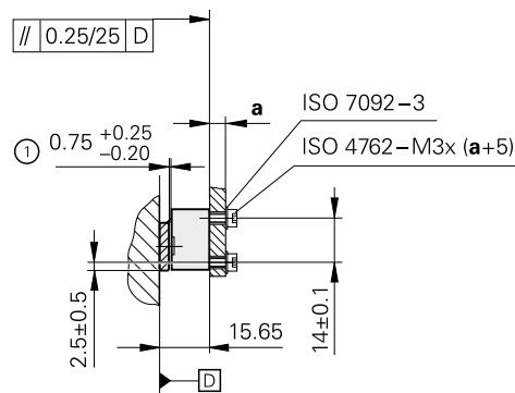
① = Mounting clearance between the scanning head and graduation
