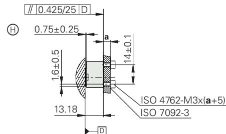
(H) = Mounting clearance between the scanning head and scale tape carrier (LIC 3107), scale tape (LIC 3109)
