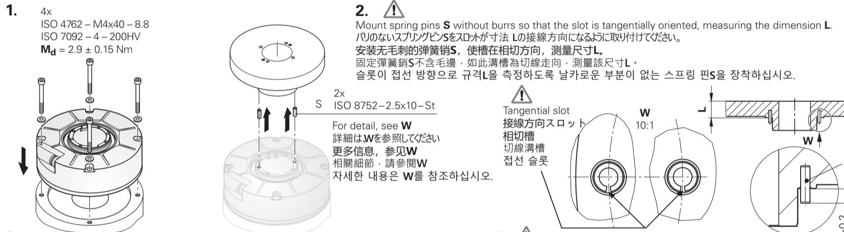
**Caution:** Pay attention to the position of the spring pins with respect to the spring pin holes **C**.
