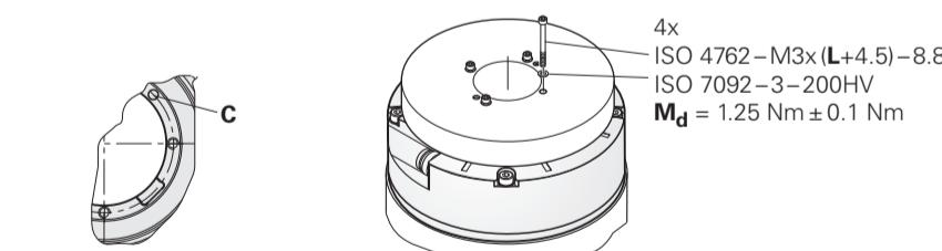
**Shaft coupling with ring nut [R] (without mechanical fault exclusion)**
