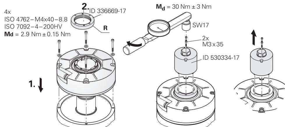
**Front-end shaft coupling (without mechanical fault exclusion)**
