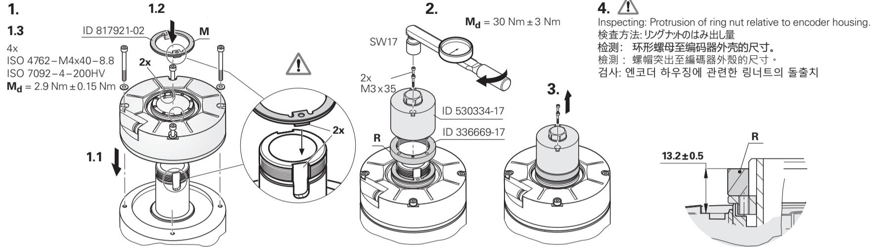
**Front-end shaft coupling (with mechanical fault exclusion)**
