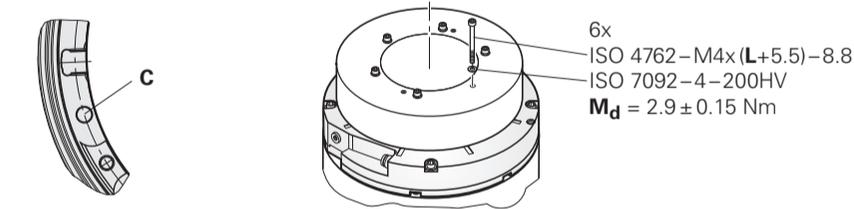
**Shaft coupling with ring nut [R] (without mechanical fault exclusion)**
