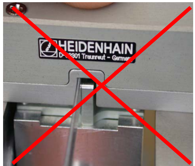
Figure 16b: Incorrect position of the spacer foil
