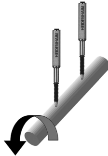
Calibrating two points on a rod.
