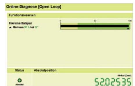
Screen showing the valuation numbers as functional reserves (e.g. with ATS software)
