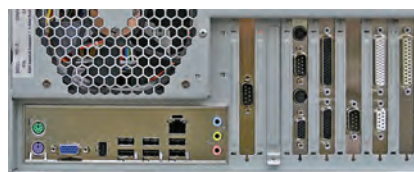
Typical PC card and flyout connectors at the rear of a PC
