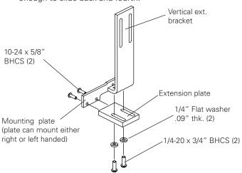
► Temporarily attach the bracket assembly to the reading head for locating purposes.
