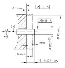
mm Tolerancing ISO 8015 ISO 2768 - m H < 6 mm: ±0.2 mm
