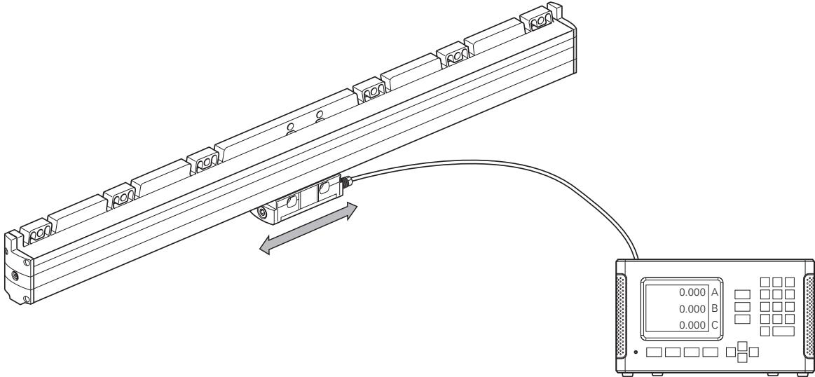
Connect the encoder to a HEIDENHAIN PWM 20/PWM 21 phase meter or other suitable subsequent electronics and check for proper function over the entire range of traverse.
