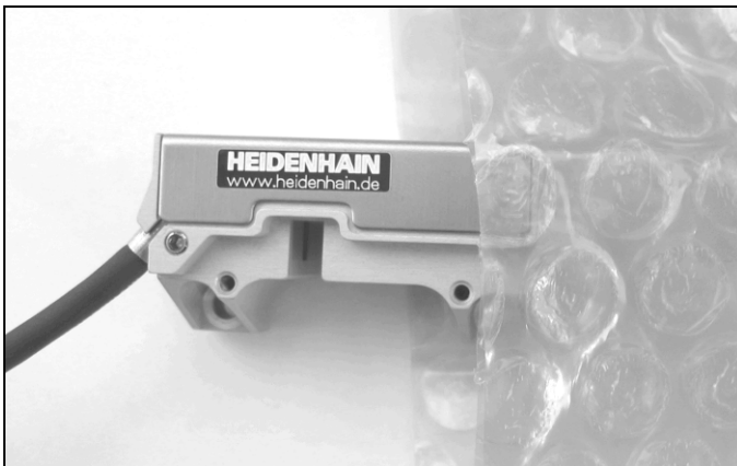
Figure 9: Scanning head with shielding bag
