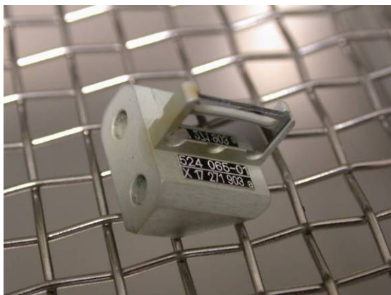
Figure 25: Scale in a basket in the ultrasonic cleaning bath
