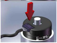
Remove test cable and install cover. Install cable assembly.
