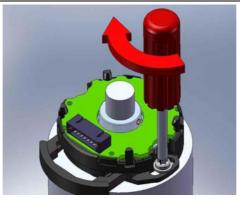
Install mounting screws finger tight, then torque to 0,21 ± 0,03 Nm (35-40 oz-in).
