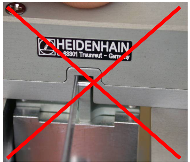
Figure 14: Incorrect position of the spacer foil
