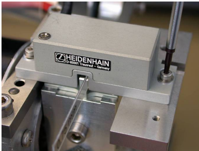
Figure 15: Securing the scanning head
