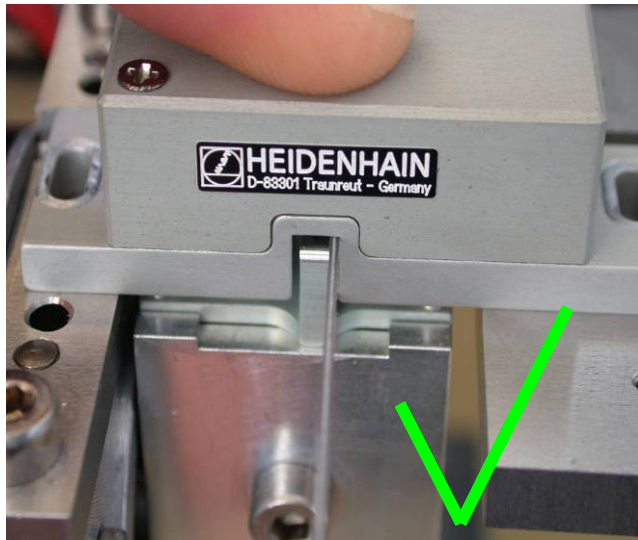
Figure 13: Correct position of the spacer foil
