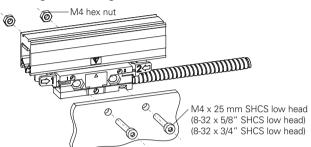
⚠ Do not tighten prior to adjusting leveling set screws.
