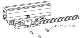
Adjust the leveling set screws as follows:
