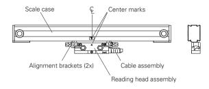
Align the center marks on the reading head and scale assembly by sliding the reading head and brackets along the scale.
