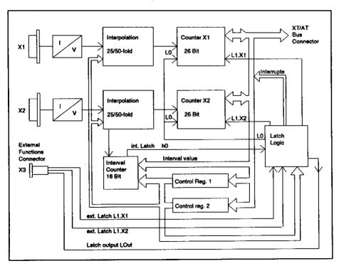
The interpolation electronics included on the IK 120 generates up to 200 counts per input signal period. This results in a finest measuring step of 1/200th part of the signal period.
