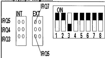
Only one interrupt signal, either internal or external, can be assigned on the board.
