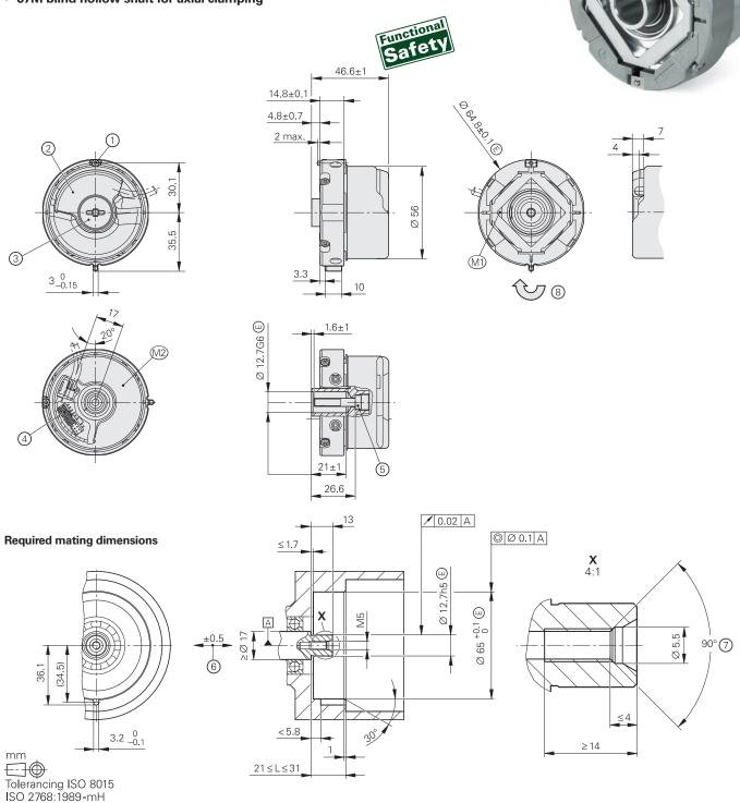
M1 = Measuring point for operating temperature
