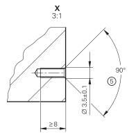
mm ----Tolerancing ISO 8015 ISO 2768:1989-mH ≤ 6 mm: ±0.2 mm
