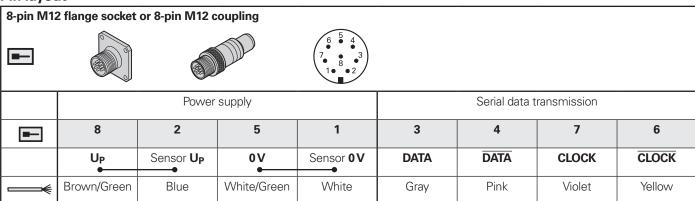
Cable shield connected to housing; U<sub>P</sub> = Power supply voltage
