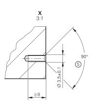
Tolerancing ISO 8015 ISO 2768:1989-mH ≤ 6 mm: ±0.2 mm
