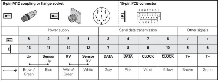
Cable shield connected with housing;  $U_P$  = Power supply; T = Temperature
