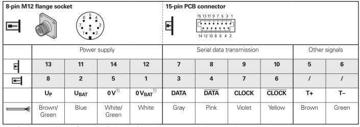
$\mathbf{U_P}$  = Power supply;  $\mathbf{U_{BAT}}$  = External buffer battery (false polarity can result in damage to the encoder)
