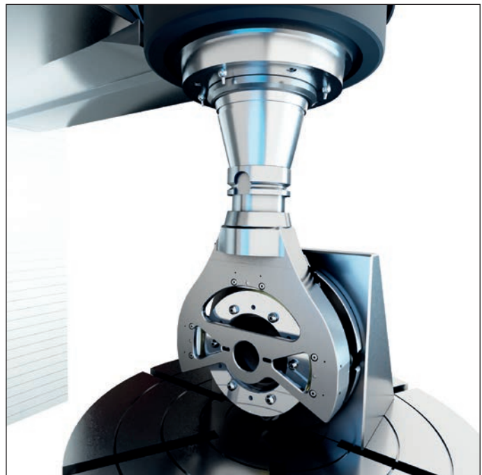
Sample mounting scenario for the RVM 4280
