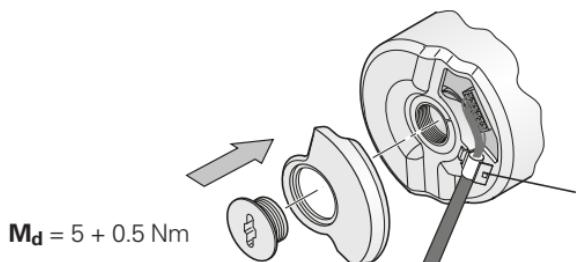
External shield on crimp sleeve
