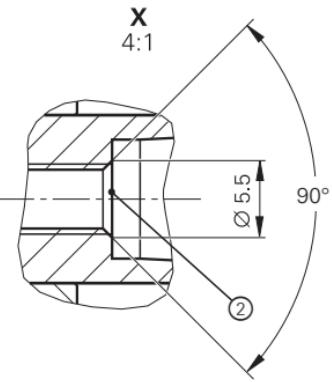
2 = Chamfer is obligatory at start of thread for materially bonding anti-rotation lock.
