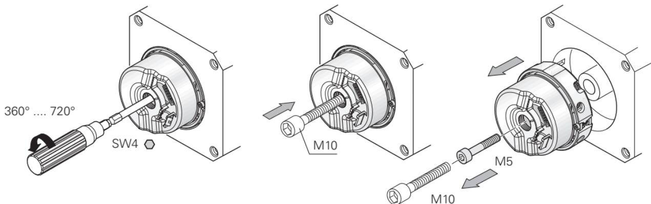
Turn the **M10** screw only far enough in to release the taper shaft.
