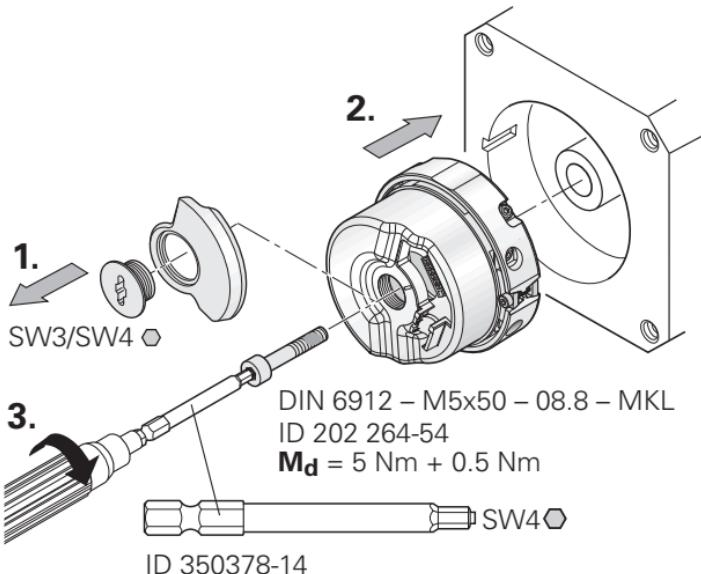
Mounting surfaces, mating shaft with thread and central screw must be clean and free of grease.
