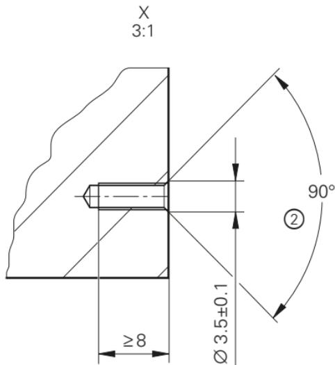
② = Chamfer is obligatory at start of thread for materially bonding anti-rotation lock
