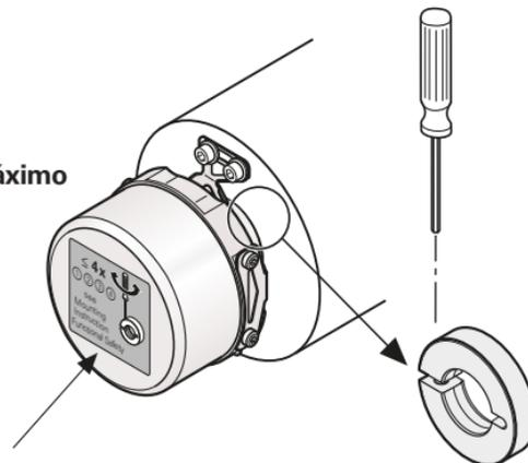
Every time the clamping ring screw is tightened, it is to be documented with a mark on the sticker. The sticker is to be applied, for example, to the encoder (see Fig.).
