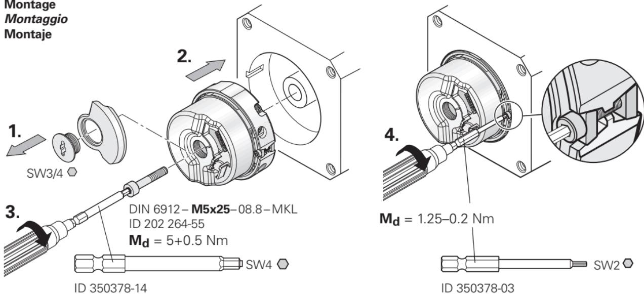
Mounting surfaces, mating shaft with thread and central screw must be clean and free of grease.
