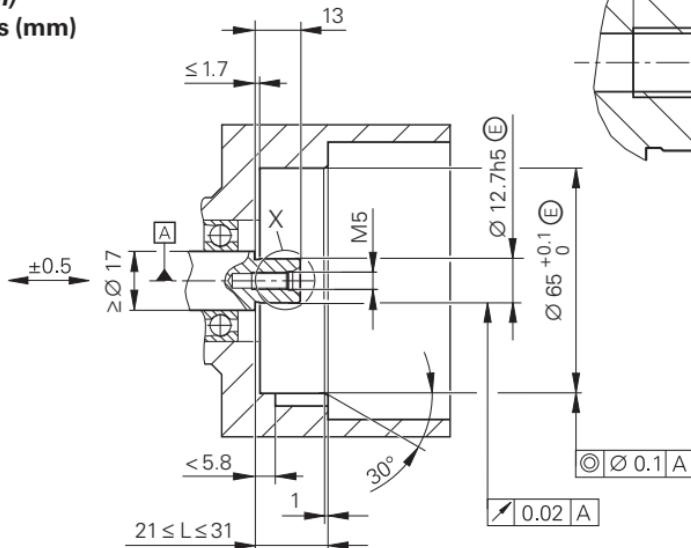
2 = Chamfer is obligatory at start of thread for materially bonding anti-rotation lock.
