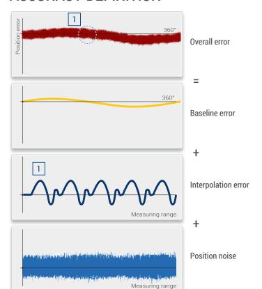
The accuracy of an encoder is mainly determined by the baseline error of the scale unit, the interpolation error of the optoelectronic scanning and the position noise.
