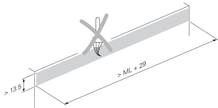
Mount the aligning rail.
