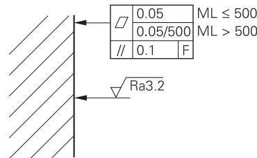
The mounting surface must be free of paint, dust, or grease.
