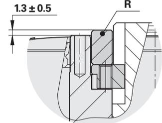
**Front-end shaft coupling (with mechanical fault exclusion).**
